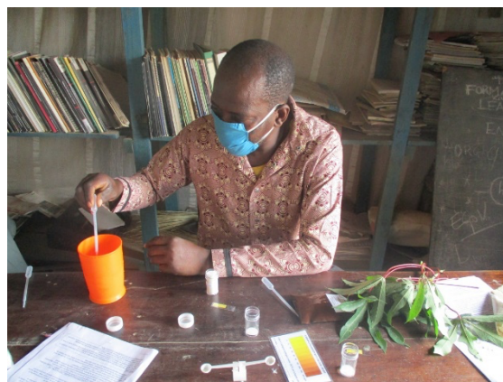
Aaron Kalala is testing cassava flour and leaves using Kit test from CCDN
